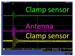
Clamp sensor (Clipping GND cable)
