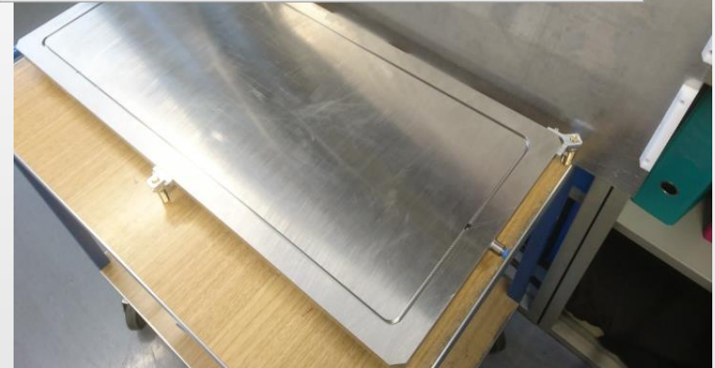
Establishing the film production facility equipped with 9 gel pouring tables
