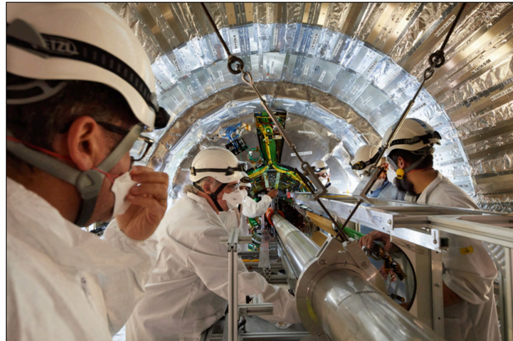
Delicate surgery: The new Pixel Tracker being installed at the heart of the CMS detector. (Photo: Max Brice/CERN)
