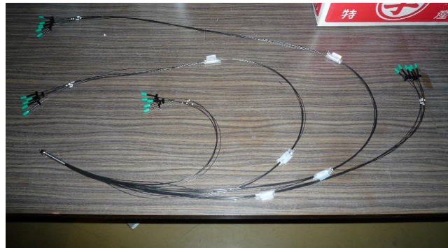
Optical fiber cables (22 fibers to a LED)
