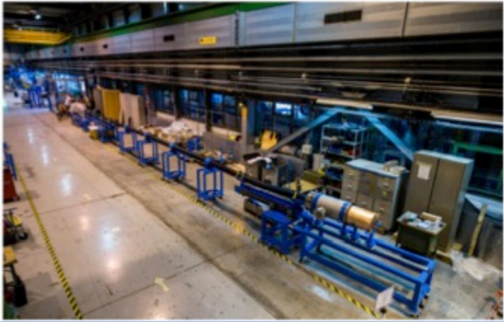
SC Link at CERN: 20 m length, up to 20 kA
