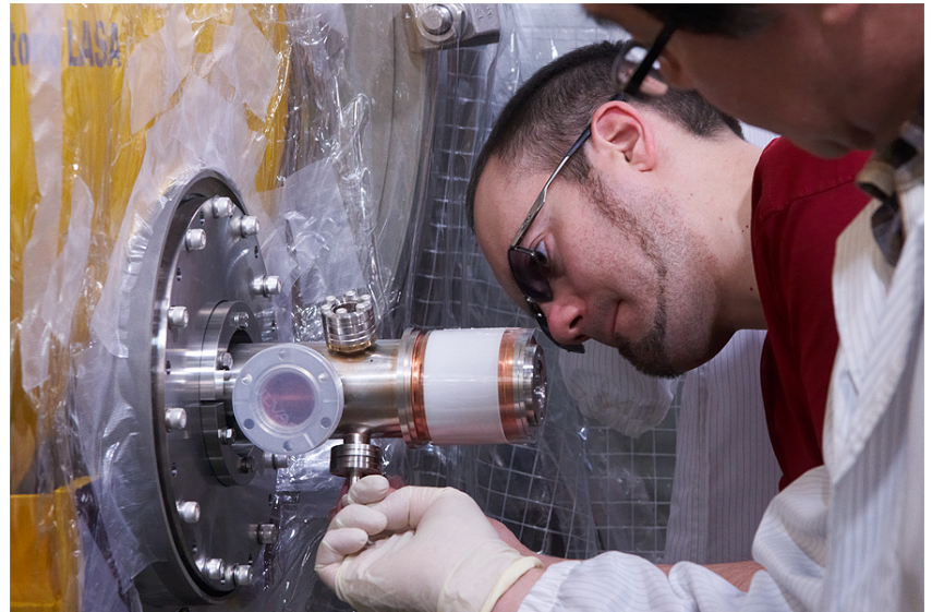
Denis Kostin from DESY installed warm couplers
