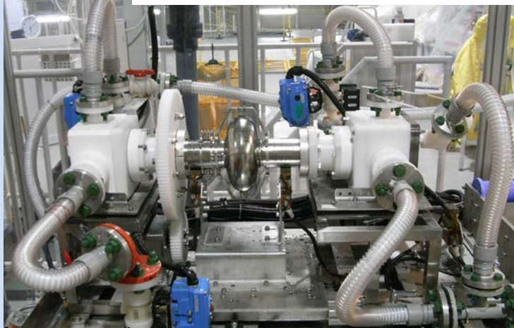
Process monitoring by Coupon on single-cell cavity
