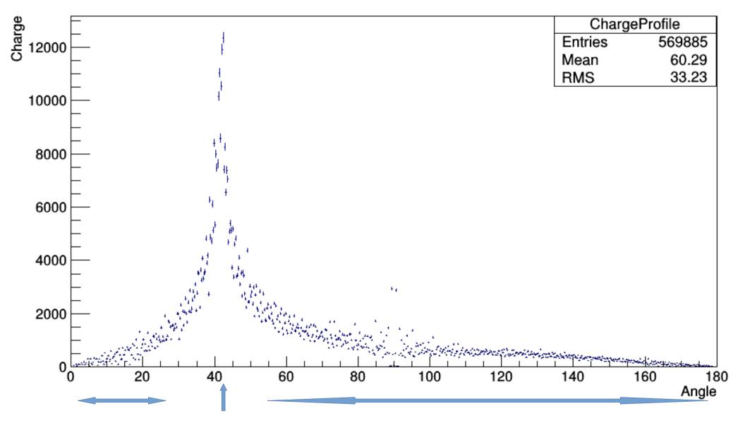
**Expectations for mPMT:** the peak will be at the same value of angle, but it will be lower along axis Y, because not all photons hit small PMT. A lot of photons hit gap between PMTs.
