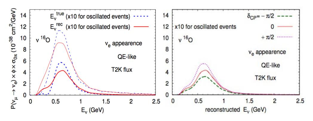
If ignored, this could lead to a wrong fit for the oscillation parameters!!!
