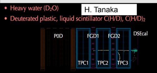
Deuterated plastic,  $D_2O$ , liquid scintillator to get at fundamental cross sections
