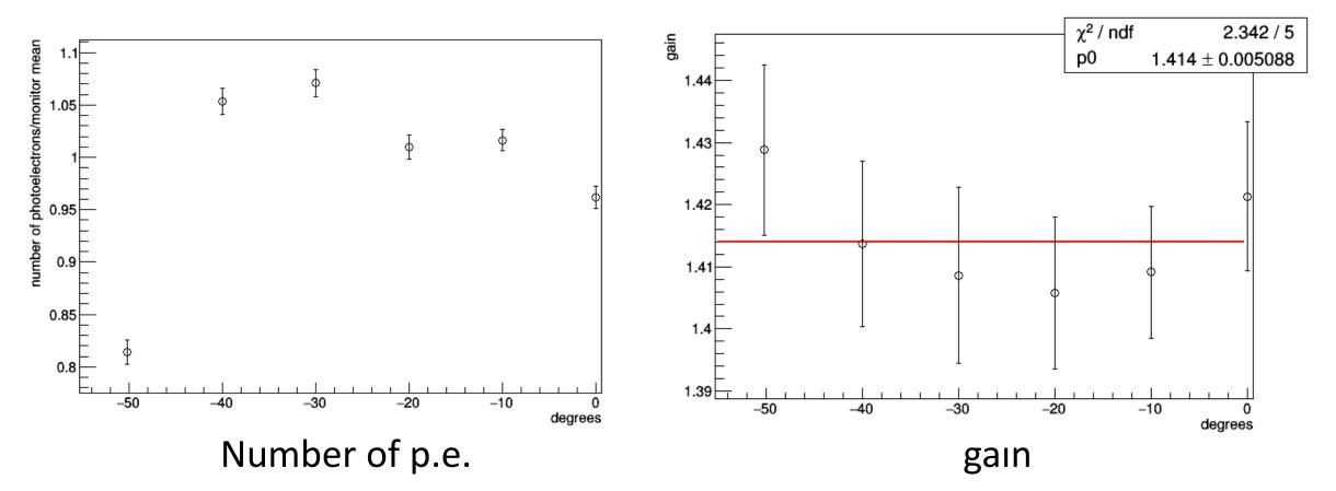
The efficiency dropped at -50 degrees. Gain is almost uniform.
