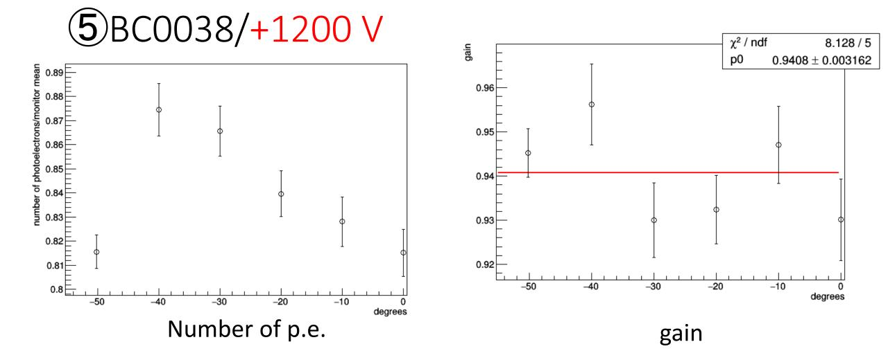
The efficiency dropped at -50 and 0 degrees. Gain is almost uniform.
