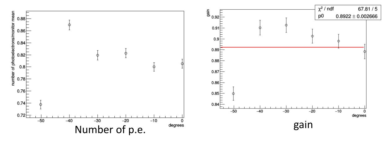
The efficiency and the gain are smaller at -50 degrees.
