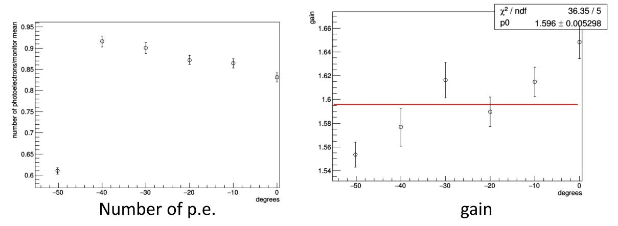
The efficiency dropped at -50 degrees. Gain is smaller at larger angles.
