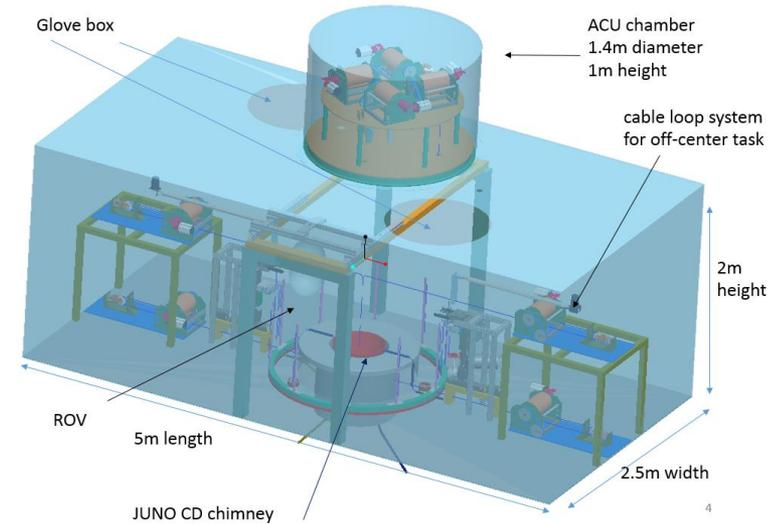
Redundant calibration system
