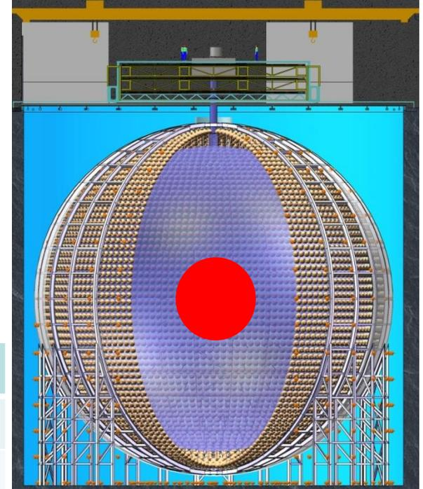
Insert a balloon filled with  $^{136}\text{Xe}$ -loaded LS(or  $^{130}\text{Te}$ ) into the JUNO detector
