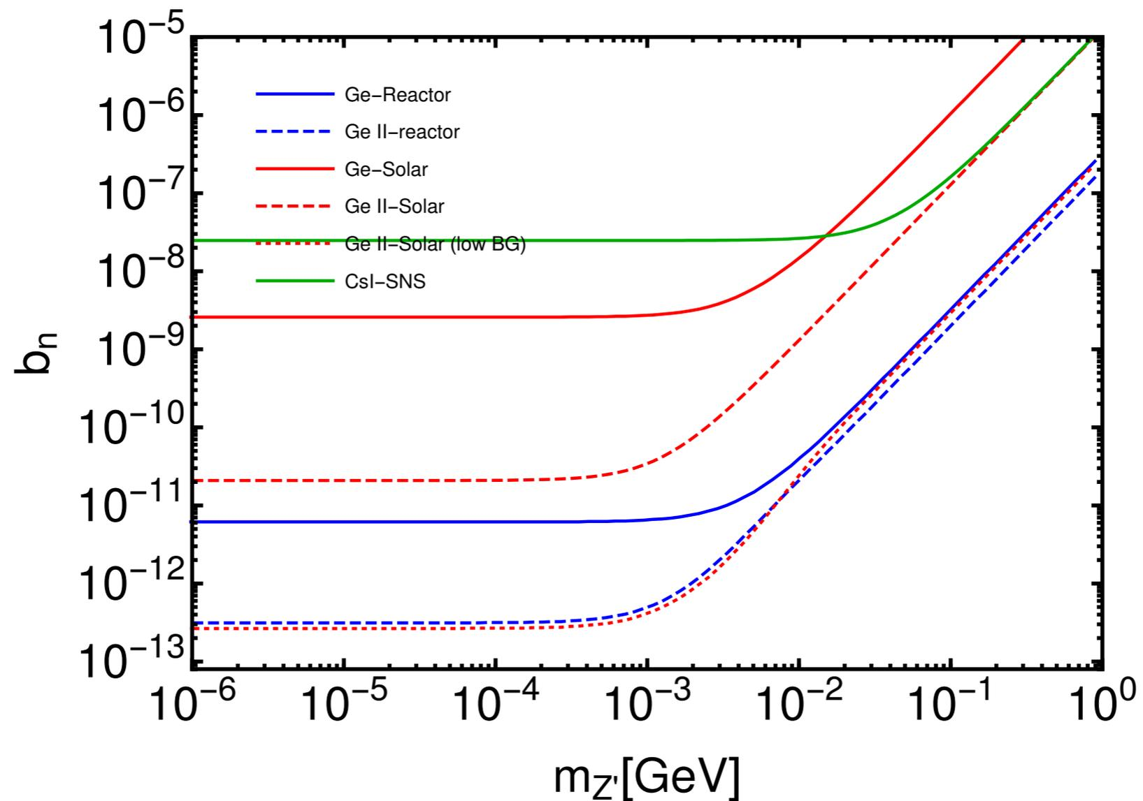
The solid blue line is 10,000 kg days in Ge with 100 dru BG and 100 eV threshold
