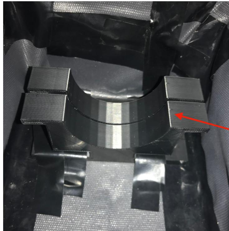
holder made by 3D printer
