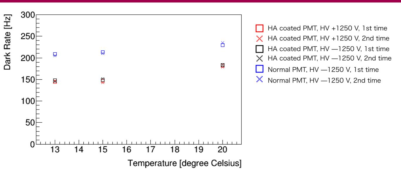
The dark rate of a normal PMT with negative HV is higher than that of a HA coated PMT.
