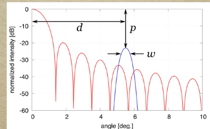
$$\left(\frac{d}{7 \text{ deg.}}\right) \left(\frac{p}{0.03}\right) \left(\frac{w}{30 \text{ arcmin}}\right)^2 \leq 1,$$
