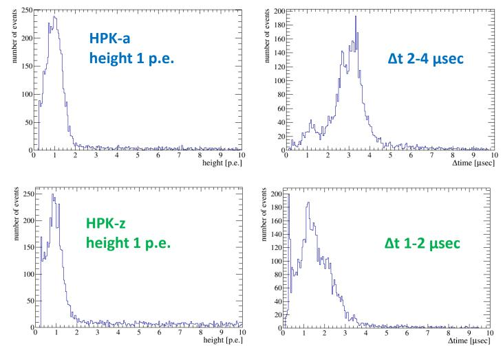
• The same 1 p.e. level signals were seen, but the time intervals between main signal and after pulse were different for 3"PMTs and another PMT.
