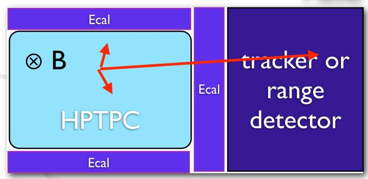
Baseline concept is 8 m<sup>3</sup> magnetised volume with ND280 micromegas readout, surrounded by ECals with tracking down stream. *This configuration must be optimised.*
