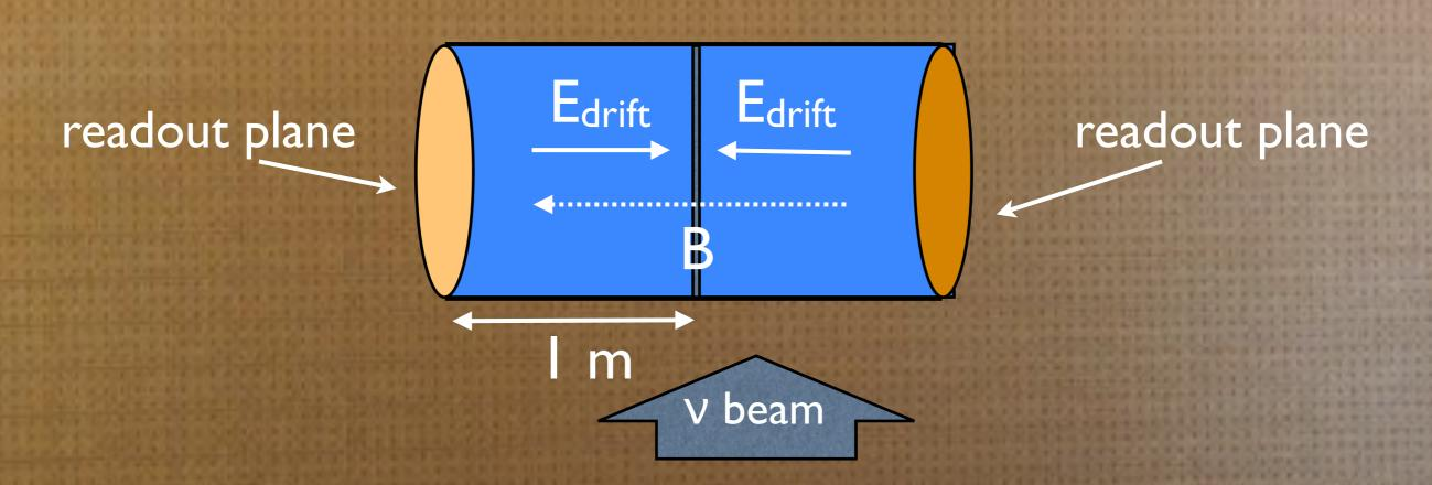
In the hypothesis of central cathode plane and contained in ND280 magnet, we will have ~ I m of drift distance
