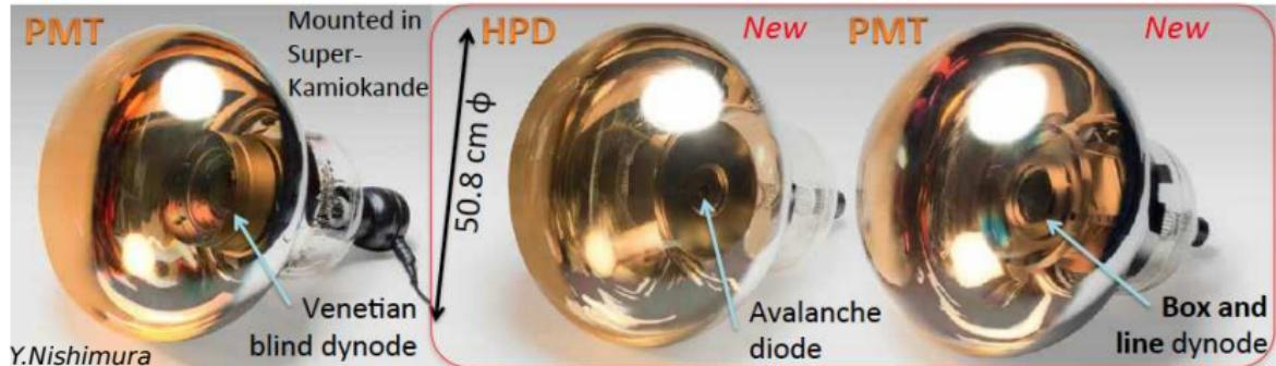
Characterize and study optical properties of PMTs under consideration for HK and near detector.
