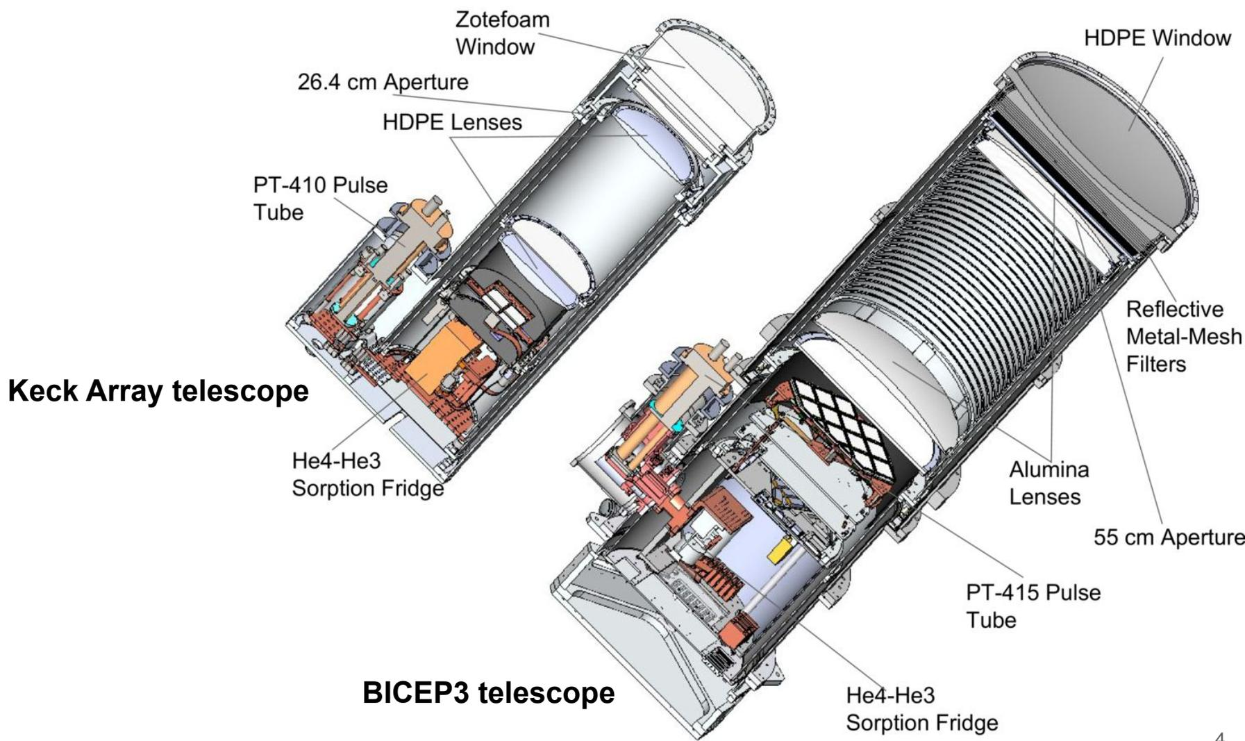
Simple on-axis cryogenic refractor with high throughput for sensitivity
