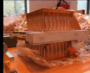
Back-to-back platelet horn array: Milano Statale (INFN) Switches: Milano Bicocca (INFN) Cavaliere et al, 2020, arXiv:2008.12721
