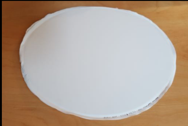
30cm diameter hot-pressed and AR-coated mesh HWP – To be cut
