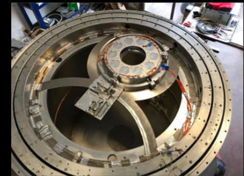
Half Wave Plate rotator: Roma La Sapienza (INFN) D'Alessandro et al, 2020, arXiv:2008.10667
