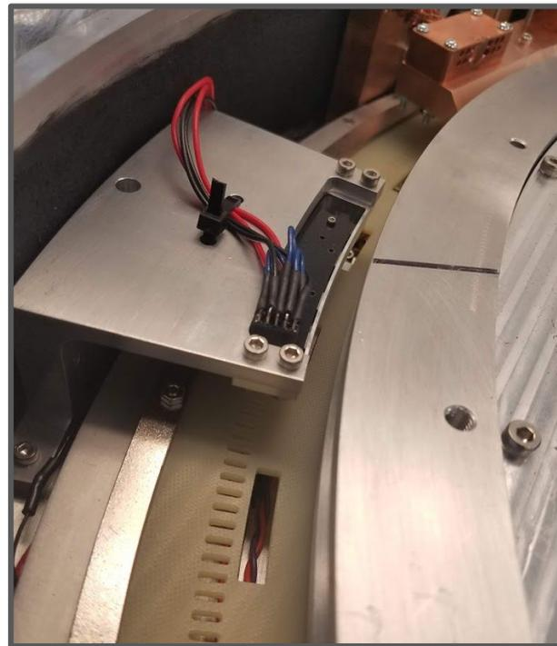
5 LED/photodiode pairs per read head with 2 redundant read heads:
