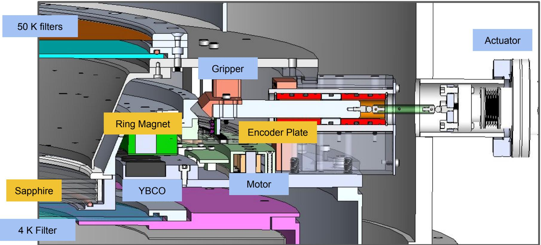
Rotor and Stator parts. In normal operating mode, the CHWP spins continuously at  $\sim 2$  Hz on a high- $T_c$  maglev bearing, carrying 3 slabs of 505 mm diameter sapphire to modulate sky polarization at 90 & 150 GHz.
