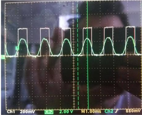
Encoder output is high SNR, square waveforms
