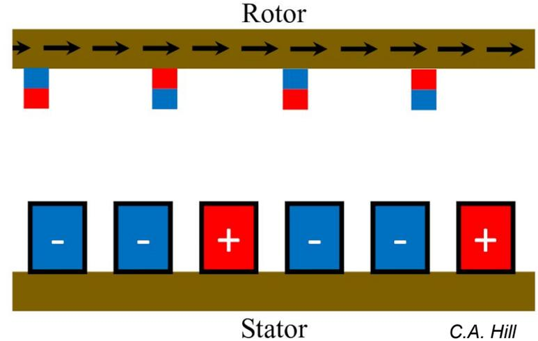
120 coils total, arranged in 3 phases, apply torque to permanent magnets on rotor rim.
