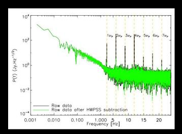
NIKA-example: continuous rotating multi-layers HWP produced a modulation also of the background signal
