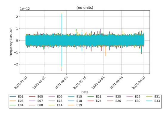
Frequency bias with removed daily linear fit after removing E02, E11, E12, E36 clocks
