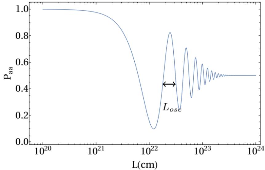
$$L_{osc} = \frac{4\pi E_\nu}{\delta m^2} \approx 20 \text{ kpc} \left( \frac{E_\nu}{25 \text{ MeV}} \right) \left( \frac{10^{-19} \text{ eV}^2}{\delta m^2} \right)$$
