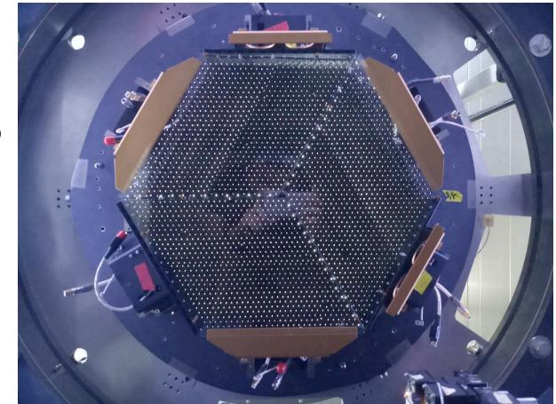
Prime Focus Instrument hosts 2394 robotic fibers on the focal plane
