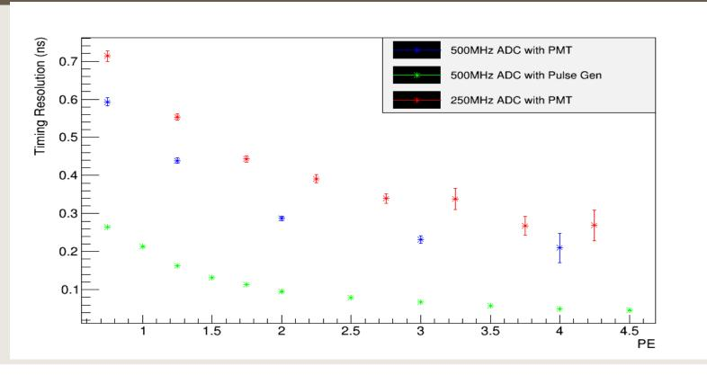
In principle the 500MHz ADC results with PMT and pulse generator should have similar timing resolution. But:
