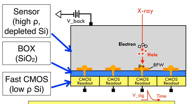
Each pixel has its own trigger logic and analogue readout CMOS circuit.
