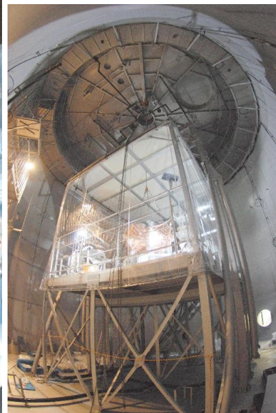
1 st LXe detector with water Cherenkov shield
