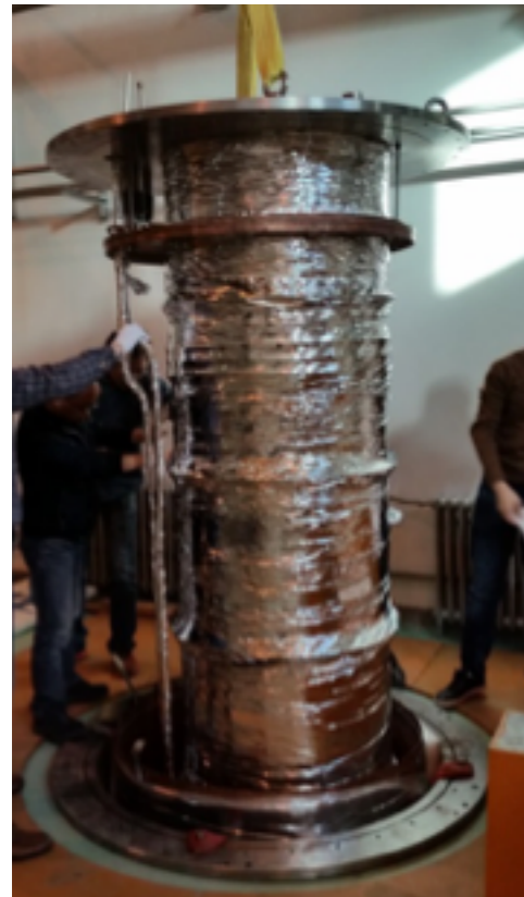
Vertical Dewar Cavity suspension Magnetic shielding
