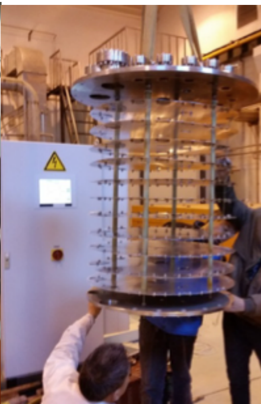
Vertical Dewar Cavity suspension Magnetic shielding
