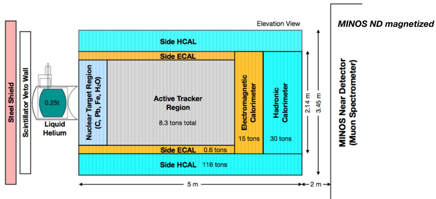
Design, calibration, and performance of the MINERvA detector
