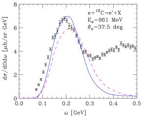
Electron-carbon cross section obtained within the IA approach using relativistic (solid line) and non relativistic (dashed line) kinematics.
