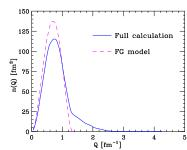
► Correlation effects lead to a quenching of the peak of the distributions and an enhancement of the high momentum tail
