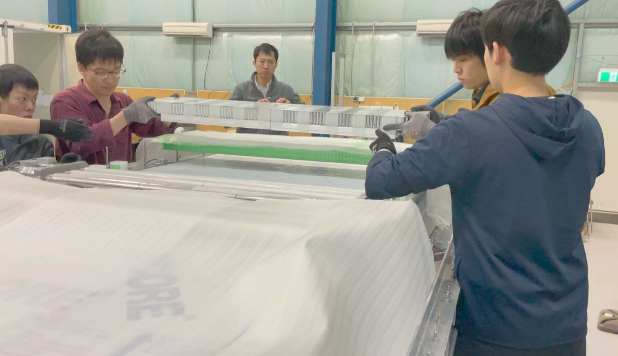
Deploying a part of Emulsion converter , 90 films in a pack, 1 m x 25 cm, 3 cm thick, 16kg
