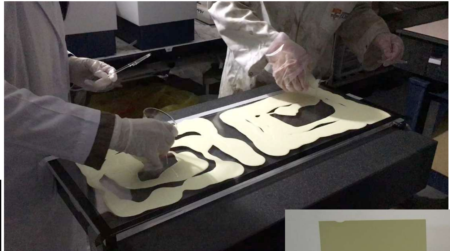
AgBr crystal formation & gel production machine
