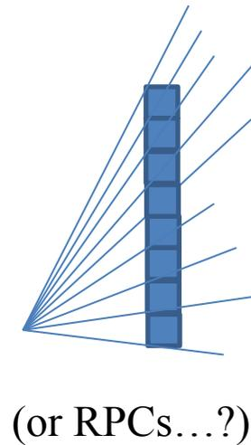
We can greatly improve the charge reconstruction of short tracks by including and optimizing a gap  $L$  between the initial few measurement planes
