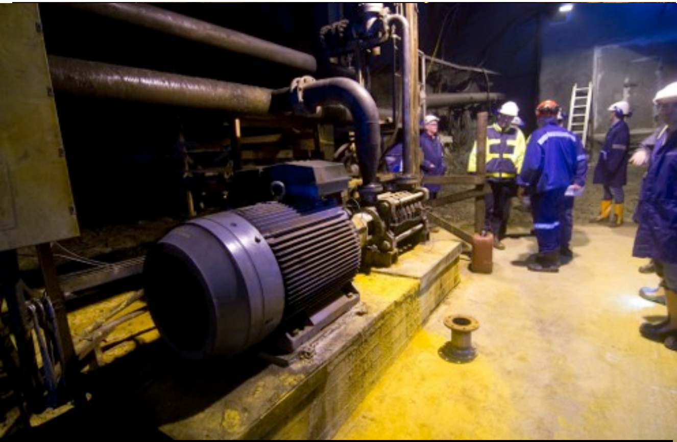
This pump alone takes all the water from 645 m to the surface
