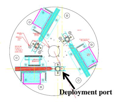
3 sources for each z axis on a turntable (position accuracy < 5 mm):
