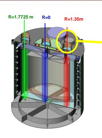
Three axes: center, edge of target, middle of gamma catcher
