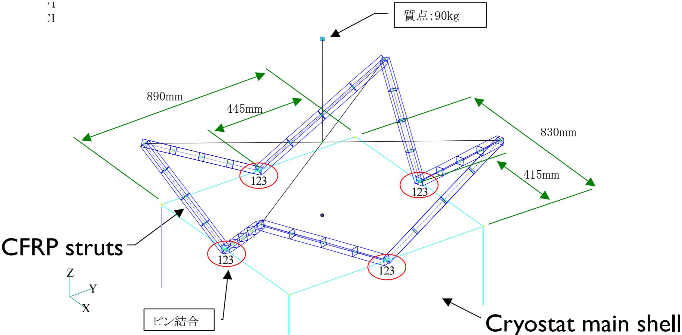
20G launch load and stiffness requirements (>30Hz lateral, >70Hz axial)
