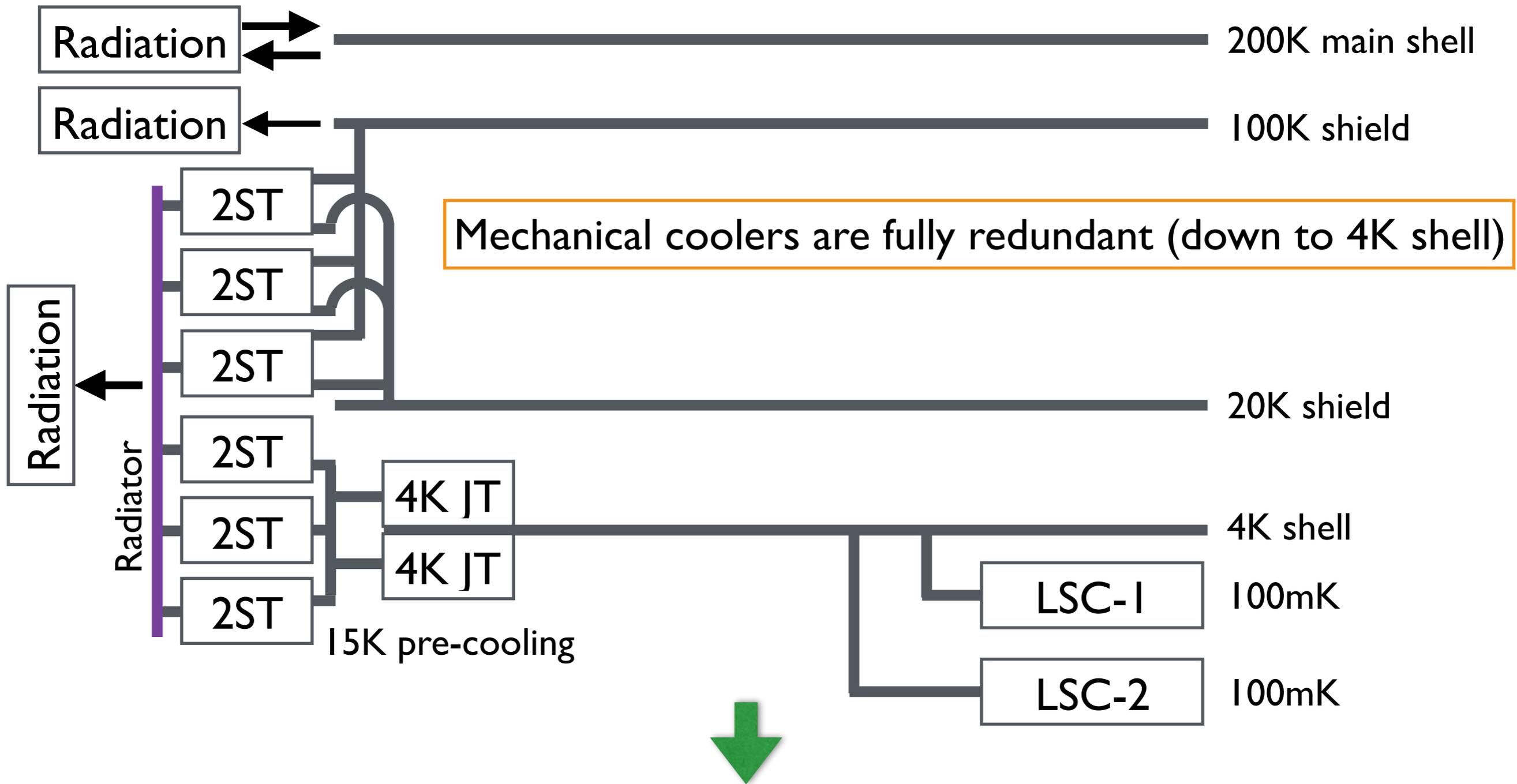
Plus margin at 4K cooling power, for ~ 220kg 4K shell mass.
