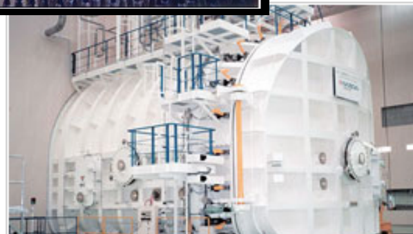
JAXA 6-m diameter space chamber
