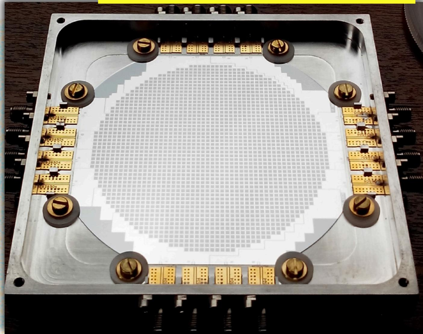
*NIKA2 thousands pixels array installed @ 30m Telescope IRAM*
