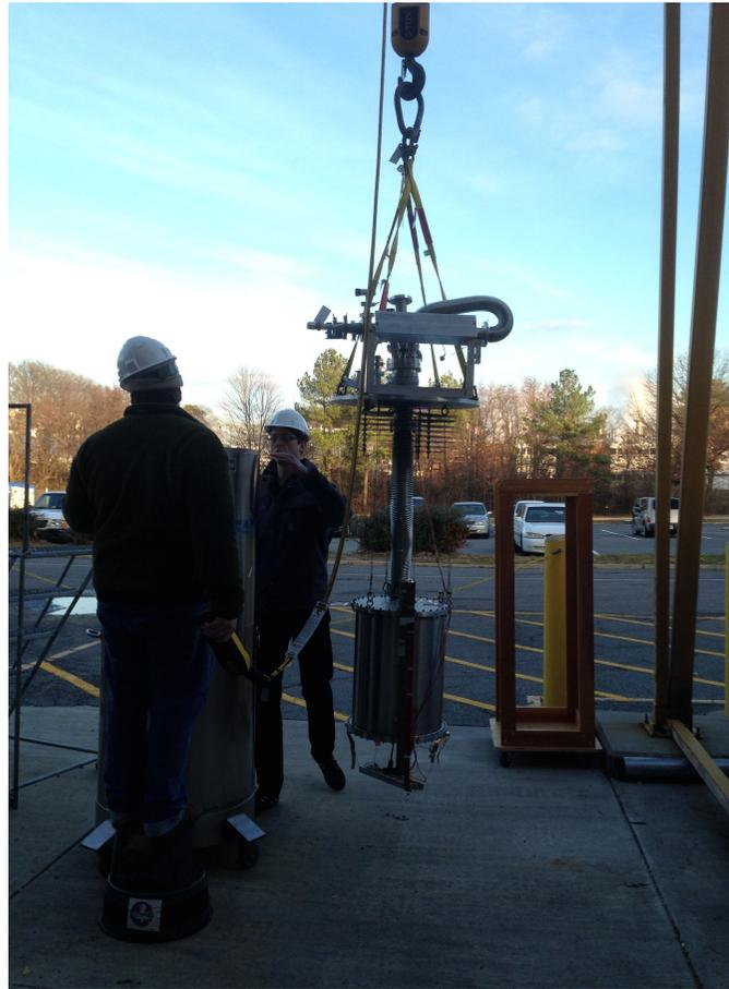
Flight camera testing in an intermediate dewar.
