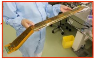
**Outermost layer of SVD** assembly downstairs
