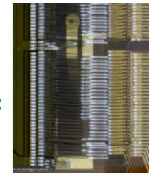
success to control the epoxy-glue viscosity under the bonding pads, which subsequently provides stable pad base.
