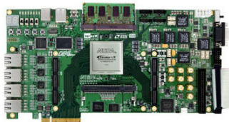
Implemented on an Altera DE4
