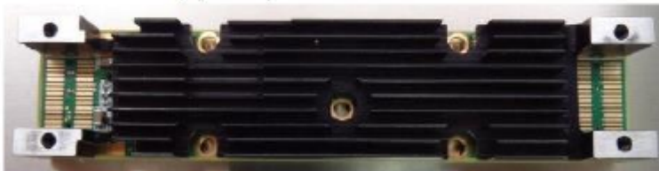
(c) A FECi with its heat sink
