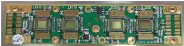
(b) Component side of a FECi
