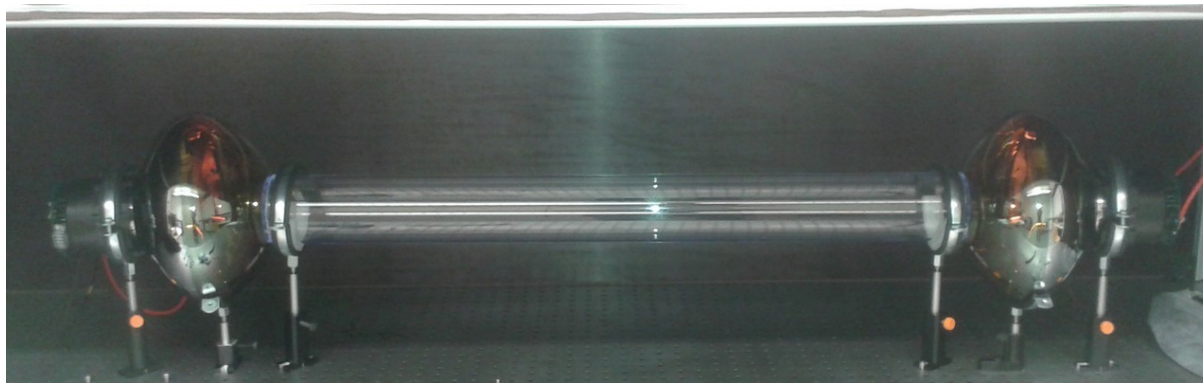
Coated tube with 2 IceCube PMTs
