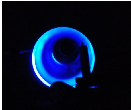
Coated tube under UV irradiation
