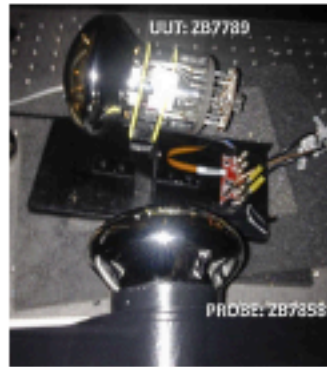
Figure 3. Left: setup where the UUT is a PMT supported by an insulating frame without any kind of coating. The PROBE is covered with insulating tape and has a dark count rate within the Vendor specifications; Middle: scheme of the setup; Right: dark count rate measured for a UUT supported by an insulating holder.
