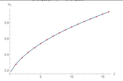
The red dots are the lattice data for the differences between adjacent charged ground states.
